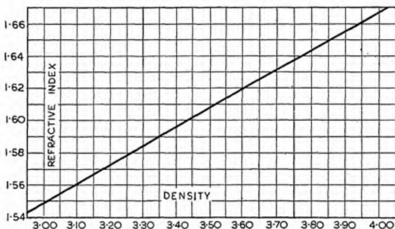
Figure 18. Graph giving relation between refractive index and density of Clerici solution
